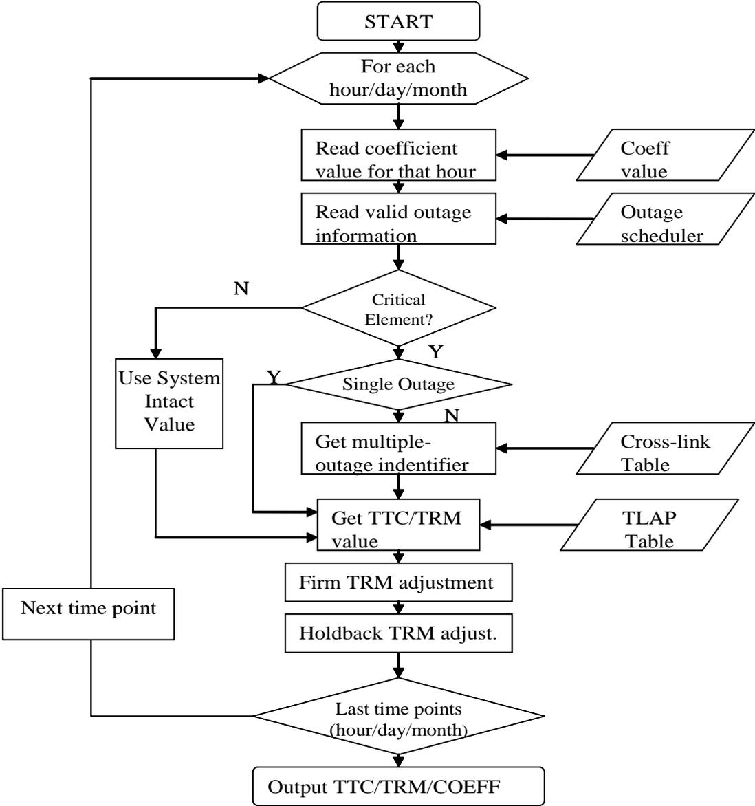
Figure 2. Process flow of the TTC/TRM calculator
